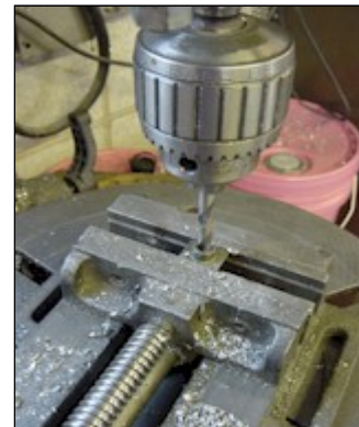
Figure 2. Drill Rear Fender Nuts
