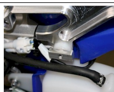
Picture #3, Coolant tank nut installation
